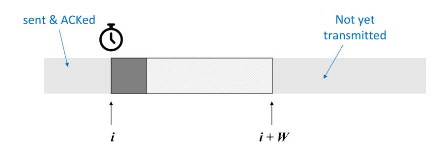
Sender maintains a **sliding** window of W **contiguous** bytes Sender maintains a single timer, for the LHS of window On timeout, sender retransmits the packet starting at *i*
