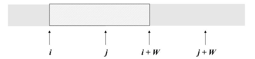
Receiver sends cumulative ACKs; sender counts #dupACKs **Fast Retransmit**: Sender retransmits *i* when #dupACKs = 3 Sender slides window on receiving an ACK for new data (j > i)
