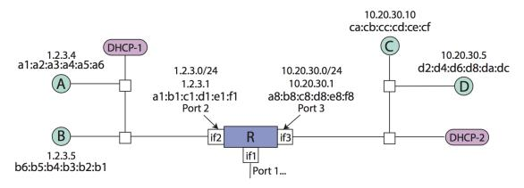
Consider the above topology. Here, two networks are connected through router R. R has three interfaces, each associated with a port, MAC address, IP address, and subnet.
