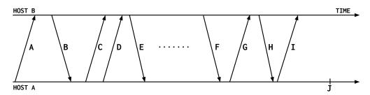
The above figure shows the life cycle of a TCP connection with normal termination - that is, connection establishment, data exchange, and teardown.
